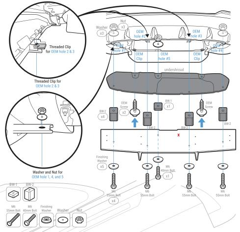
Remove the OEM Screws located under the bumper near the rear wheels to get access to the inside of the bumper
