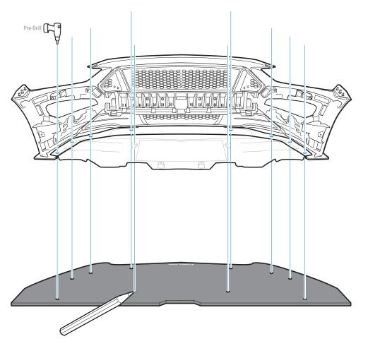
Use provided hardware to mount the Front Splitter to the front bumper
