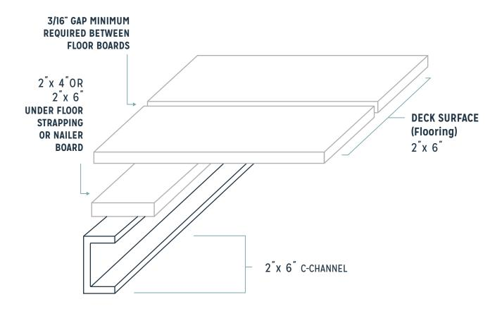
**USE B4-11.5** (FOR 2" x 4" UNDER FLOOR STRAPPING) **USE B6-11.5** (FOR 2" x 6" UNDER FLOOR STRAPPING)
