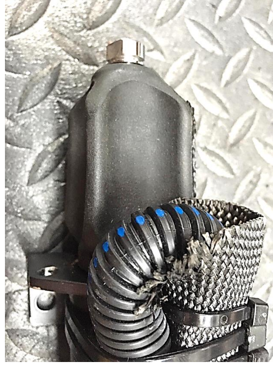
Boot is not compressed and spring can not be seen.
