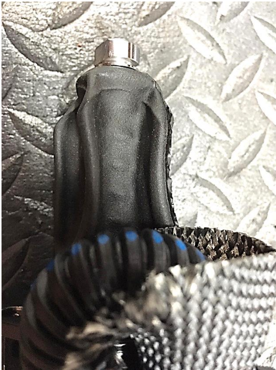
Boot compressed solenoid will not work correctly and spring can be seen.
