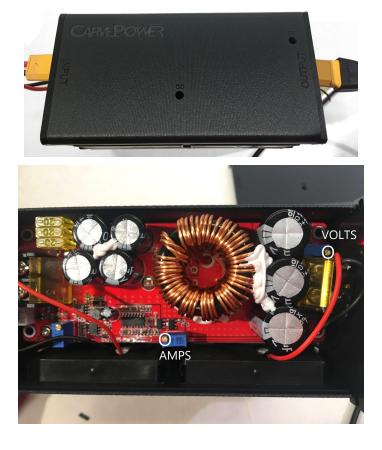
When setting the voltage, watch the output voltage display on the right side. The voltage can be slow to respond, so stop turning the screw a little bit before it reaches the target voltage.
