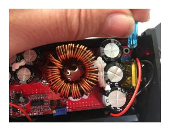
The current is set by default to 5A. This will charge a Onewheel plus in approximately 25 minutes, and is fast enough to keep up with charging while riding in most circumstances. The battery cells in a Onewheel and Onewheel+ can handle up to 10A, so 5A is safe. Charging at higher currents can reduce the lifespan of the battery, so it's best to do this only while needed in the field, and use the wall charger whenever possible.
