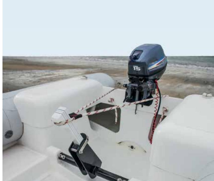
**TOP** The wheels are retracted/deployed with a simple lever mechanism, held in place by a rope stop.
