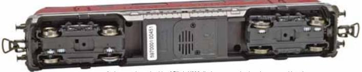
A glance at the underside of Piko's V200 discloses a speaker housing recessed into the fuel tank. Two screws on either side of the tank ends hold the chassis and shell together.
