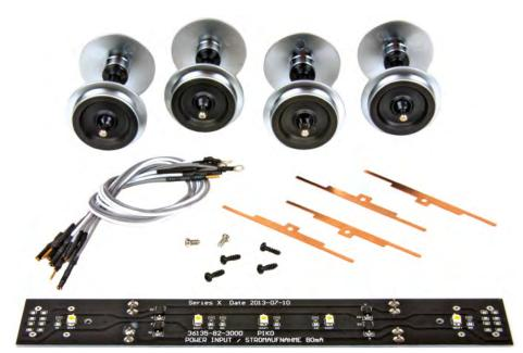
The installation of the new lighting kit for the previously reviewed Piko coach and combine is a bit more involved than that of the drover caboose. Two sets of metal wheel sets will also need to be purchased in addition to fitting the axle wiper style electrical pickups on the trucks, running the wiring up through the car body, and attaching the PCB to the underside of the roof. However, the results are worth the effort!
