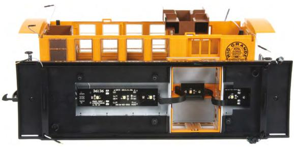
With a little careful effort, the roof on Piko's cars will snap off yielding access to the interior for the addition of figures or one of the manufacturer's LED light kits. As the drover cabooses come factory equipped with metal wheels and wire leads, its associated lighting PCBs can be installed in the car's roof in under 20 minutes. The tiny LEDs give off a warm, but bright yellowish glow that can be easily seen in a normally lit room.
