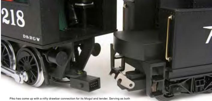
a mechanical and electrical coupling, the eight-pin, truck-mounted plug on the tender seats into the receptacle beneath the engine's cab with an outer metal bracket swinging down over the plug and grabbing onto the pins extending out from the sides of the receptacle.
