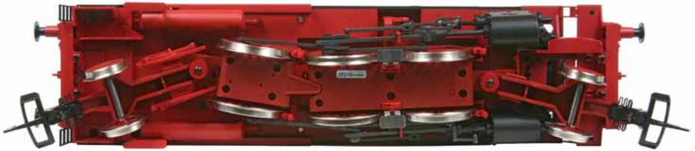
Similar to the articulation used with the previously reviewed Piko Crocodile electric locomotive, the 2-6-2T's gearbox has been divided into two segments with the motor housed along with the first two axles in the forward sealed compartment and the rear axle driven via a drive shaft in the rear section. Note also the stainless steel rims mounted on the plastic spoked drivers as well as on the Bissel style bogie (pony trucks) wheels and the truck mounted hook and loop couplers.
