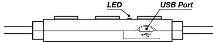
**POWER ON:** Press the
