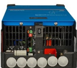
MultiPlus 2000 VA (bottom cover removed)
