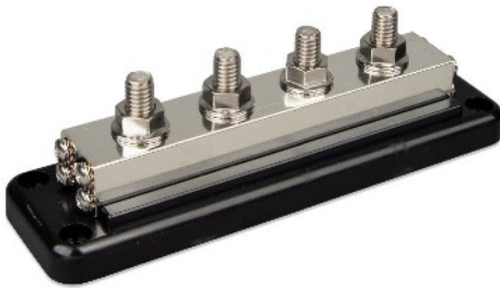
Busbar 600 A with 4 high current terminals and 8 low current screw terminals, without cover
