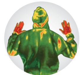
KLEENGUARD* A45 Coverall The temperature is lower and more homogeneous. The body stress for the person is considerably lower.
