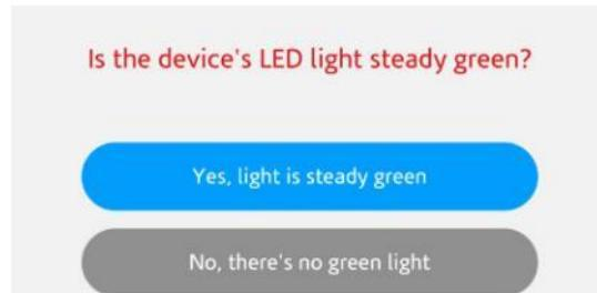
If the device doesn't have a solid green light unplug it from power and hold down the reset button for 15 seconds. Afterwards the led on the device should be steady green.
