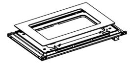
Loosen up the 5 screws on the door frame
