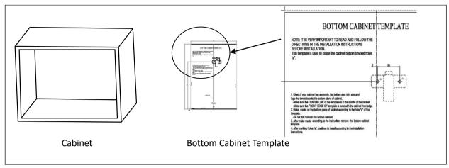
Mark the bottom panel with position "a" according to the template.
