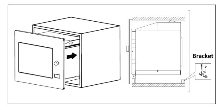
Open the door, fix the oven to the cabinet with screw, as shown in the diagram below :
