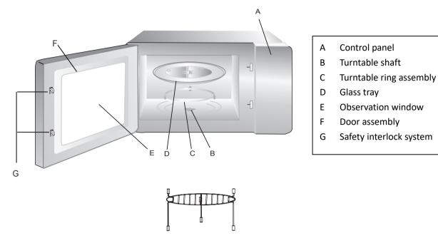
Grill Rack( Only be used in grill function and be placed on the glass tray )
