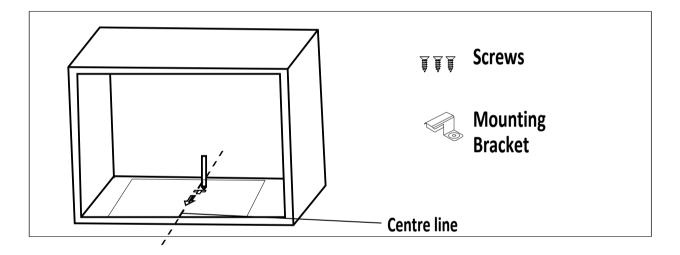
Remove the template and fix the bracket with screws.
