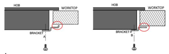
Ensure the brackets do not touch or come to rest on the cutout face of the worktop after installation.
