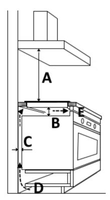
To be able to function optimally and last a long time, the ceramic cooker hob is to be installed in good a working environment. Provide for adequate ventilation as shown in the diagram beside.
