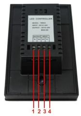
3 and 4: power input, input voltage range: 12-24V, 3 for positive, 4 for negative. 1 and 2: power output, output voltage is 12-24V, Max output current is 8A, 2 for positive, 1 for negative.
