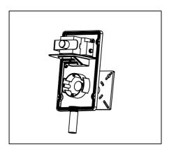
4) .After connected line, fitted with a reflector and PC cover, screw down the screws.
