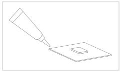
3. All ends of the section must be sealed with silicone sealant or silicone adhesive to prevent short circuits.
