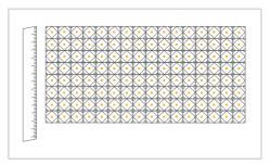
1. Before cutting the LED pixels light sheet, always measure and calculate the shape you want and check the splitting lines which show you where to cut on the LED pixels light sheet.
