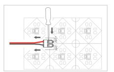
**Disconnecting:** Use awl to push down the small button on on-board connector. Then pull out the wire.
