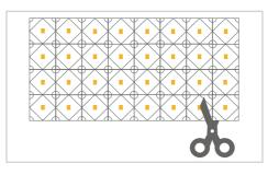
2. When cutting the LED pixels light sheet, one must cut along the split ting lines on the sheet. The electrostatic ring is needed at this step.\*DO NOT cut anywhere outside of the designated splitting lines.
