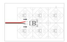
Insert the power lead wire or jumper wire into connector. Make sure to insert it **all the way in** until non of the copper core is visible.
