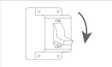
3. Always turn off the power at circuit breaker before any LED pixels light sheet installation.
