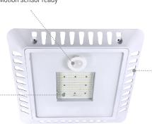
High performance, die cast heat sink transfers heat from the light engine to the environment, via large cooling fins, drawing heat away from the fixture, and extending the lifespan of the LEDs.
