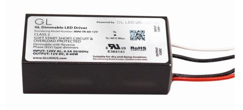
ELV (Electronic Low Voltage) dimmable drivers are compact power supplies that can be placed in remote locations, and provide stable and efficient power. Advanced technology reads the signal from a TRIAC dimmer switch for smooth dimming. They are also already derated, which means they can be loaded to maximum wattage capacity.
