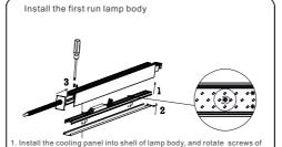
Install the cooling panel into shell of lamp body, and rotate screws of fixing card clockwise by 90° to fasten the cooling panel into the lamp;
