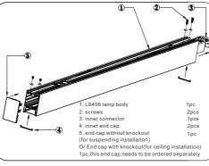
Firstly, loose the 2 screws at the lamp end, and pull out the inner connector from the lamp body, then fix the inner connector by 2 screws again. After finishing the wiring connection(see the steps on the continuous connection).fix the end cap by screws and insert the inner end caps at both
