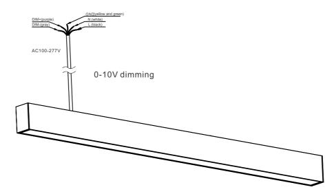
(Remark: The max current consumption of our driver to 0-10V dimmer is 2mA each one)
