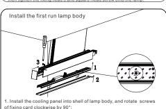
of fixing card clockwise by 90°; 2. Press and mount the PC cover and inside cover plate on lamp;
