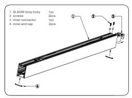
loose the 2 screws at the lamp end, and pull out the inner connector from the lamp body, then fix the inner connector by 2 screws again, insert the inner end caps at both sides.
