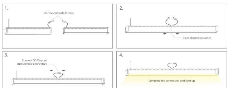
This approach simplifies installation and protects LED strip lights from potential damage. On the other hand, extra efforts may be needed to avoid a less tidy appearance with visible connectors.
