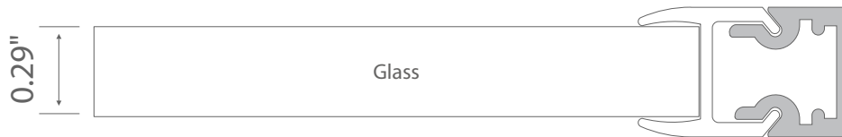
Installing with 0.29in glass
