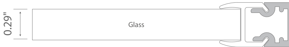
Installing with 0.29in glass
