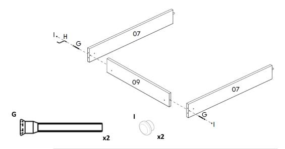
Note: use the allen key (H) to adjust the structural screws (G).
