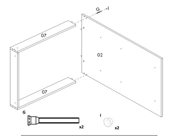
Note: use the allen key (H) to adjust the structural screws (G).
