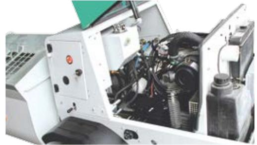
3-cylinder, liquid-cooled diesel engine that
