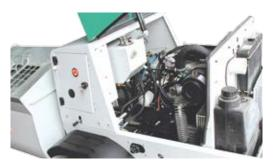
3-cylinder, liquid-cooled diesel engine that meets the latest EPA regulations and reduces noise. 2400 rpm operating speed for less wear and low fuel consumption.
