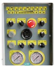
Anti-vibration control panel with electromechanical controls (Standard hour meter)
