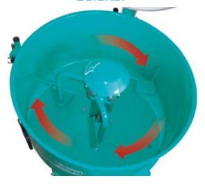
The paddles are always in the mix, working hard. Even stiff muds are mixed thoroughly and completely.
