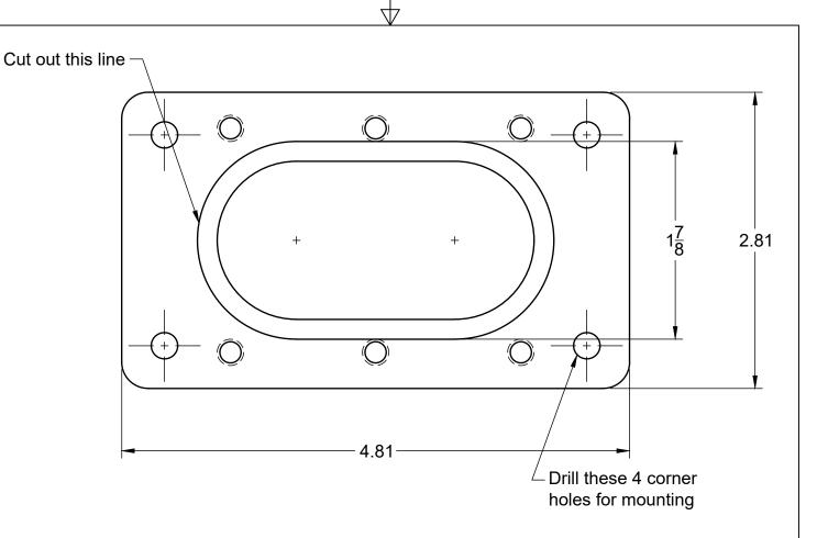
Make sure your printer is set to print at 100% scale and double check the dimensions match the printed size. Mark the centers of the oval and the 4 corner holes using the template and a center punch. Use a 1  $_{7/8}$  in hole saw to cut these out and then cut the straight lines between them to make the oval. We recommend an air saw but a Sawzall or cutoff wheel will also work. The 4 corner holes get drilled out to  $_{5/16}$  in, we recommend using a step drill for this.
