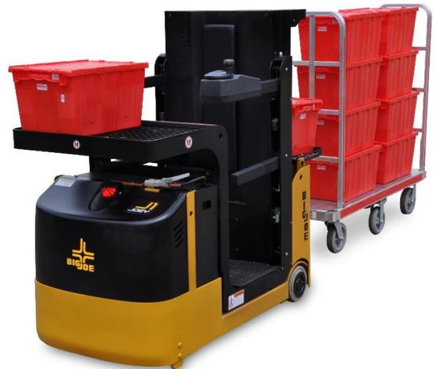
The Joey can turn in as little as a 72" aisle, lift an operator up to 162", and transport up to 3,000 lbs.
