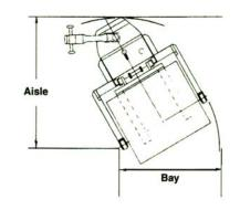
Note: Aisle dimensions listed above assume the bay width to be straddle OD plus 2" (1" on each either side of straddle leg). Straddle OD is the load width plus 10"
