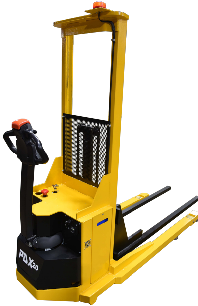
PDX20 customized with extended forks and straddles for furnace loading operations.
