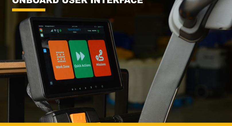
The Pallet Mover AMR features an easy to learn user interface accessed via the onboard touchscreen, allowing you to set-up, map and start missions in less than one hour. If you can use a smartphone, you can program the Pallet Mover AMR!
