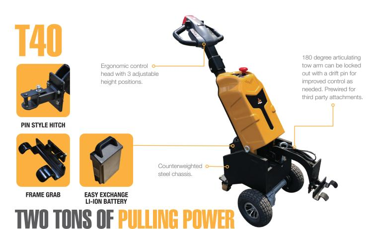
**Built to move your heaviest loads.** The T40 was designed to take on loaded carts and large mobile loads weighing up to 4,000 lbs. It can reduce physical strain and potential injury risks while freeing up other more expensive equipment like riding forklifts to perform the tasks which they were intended for, instead of towing carts from place to place. The T40's S2 60 minute rated electric drive motor with heavy duty transaxle housing delivers plenty of torque to move loads with confidence.
