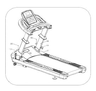
1. Fix the left and right motor side covers (13、14) to the motor top cover (11) with screw ST4.2\*12 (96) by using Phillips screwdriver (81).
