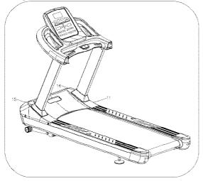
1. Fix the Left and right upright tube covers (15, 16) to the motor top cover (11).
