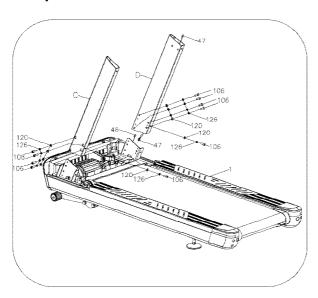
1.Fix the left and right upright tubes (C, D) to the main frame (1) with bolt M10\*20 (106),spring washer (126) and flat washer (120) by using 8#Allen wrench (79).
