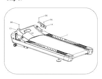
1.Lift up the left and right motor side covers (13 \, 14) by using Phillips screwdriver (81) and ST4.2\*12 screw (96).
