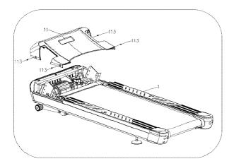
1. Disassemble bolt M6\*12 (113) by using 5#Allen wrench (80), remove the motor top cover (11).
