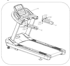
1. Fix the left and right handle bar (E $_{\times}$ F) to the console (A) with bolt M8\*15(133) and washer (124) by using 5# Allen Wrench (80).
