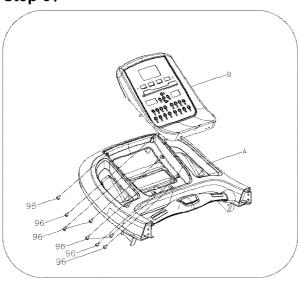
1. Fix the console panel (B) to the console top cover (A) with screw ST4.2\*12 (96) by using the Phillips screwdriver (81).
