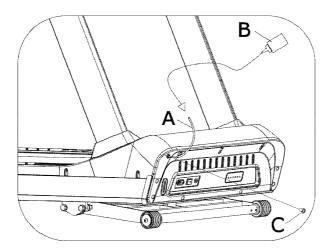
After you finish the adding of oil, please insert the plug C back, press STOP button and hold on about 3 seconds under standby mode, the oil indicate light will be off.
