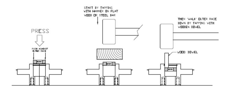
INSTALLING NEW BEARINGS
