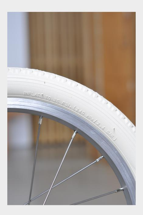
Using a bike pump that is compatible with Shrader valves, pump the tires to a max of 35 PSI.
