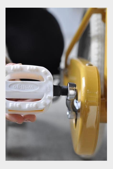
Thread in the right and left pedal. The pedals are marked with either an "R" or an "L"—the right side of the bike is the "drive" side or the side with the chain.
