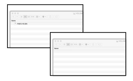
4) It will take about 30 seconds for the firmware to install. Once firmware install is complete, the COUNTcam 2 folder will reappear on your computer. Delete the 'FIREFLY6.BIN' file, then eject the COUNTcam 2. If the COUNTcam 2 folder reappears immediately, the install was likely unsuccessful, start from step 1 and attempt to install the firmware again.
