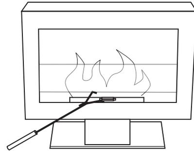
The curved ends in the handle provided (Part J) will fit into the holes in the lid of the burner. You can adjust the flame height to get the desired flame height and heat output. When you are ready to extinguish the fireplace, use the handle to slide the lid of the burner completely closed over the opening to cut off the oxygen supply to the fuel. This will snuff out the flame.
