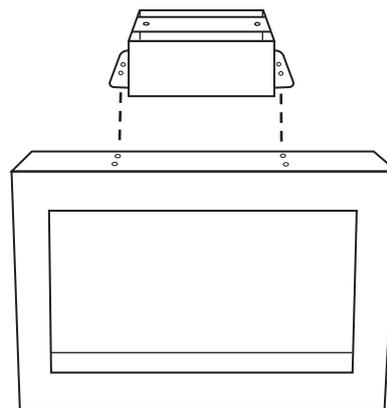
Turn your fireplace upside-down onto its top and place the stand (Part H) onto the fireplace. Make sure the flanges that stick out line up with the 4 holes pre-drilled in the fireplace.
