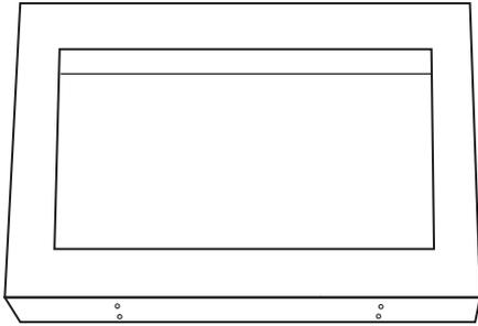
Take fireplace frame (Part A) out of plastic bag and lay the backside onto a carpet or towel with opening facing up.
