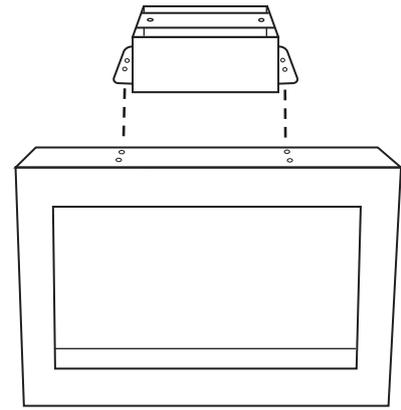
Turn your fireplace upside-down onto its top and place the stand (Part H) onto the fireplace. Make sure the flanges that stick out line up with the 4 holes pre-drilled in the fireplace.
