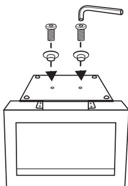
Insert plastic washers (Part L) into the holes on the glass base (Part I) and secure the glass base onto the stand using the thick .75" screws (Part M) using the hex tool provided. Be sure not to over tighten. Until screws are secured, glass may not be stable. Be careful and insure that glass base does not fall before securing.
