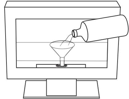
Using the funnel provided, (Part N), carefully pour in the liquid ethanol fuel for fireplaces into the burner about  $\frac{3}{4}$  full. Make sure you do not over fill the burner. If any fuel does spill, you should always wipe it up prior to lighting your fireplace.
