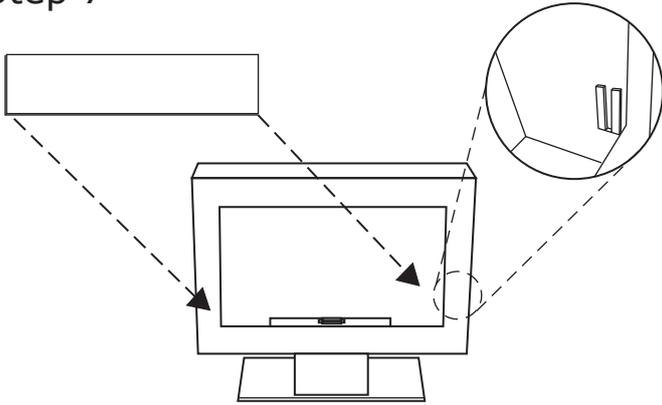
Insert glass panel into the slots located on the inner sides of the fireplace.
