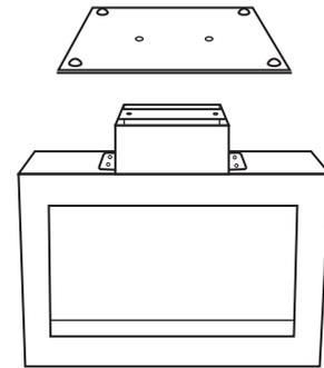
Now place the black glass base (Part I) over the stand so that the holes in the glass line up with the holes on the bottom of the stand. Make sure the rubber feet on the glass base are facing you. This will become the bottom of the fireplace.
