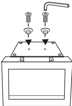
Insert plastic washers (Part L) into the holes on the glass base (Part I) and secure the glass base onto the stand using the thick .75" screws (Part M) using the hex tool provided. Be sure not to over tighten. Until screws are secured, glass may not be stable. Be careful and insure that glass base does not fall before securing.
