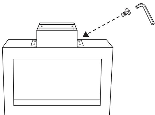
Attach the stand to the fireplace frame using the 4 .5" screws (Part K) using the provided hex tool.
