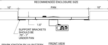
SPARK IGNITION BY AA BATTERY MATERIAL: 304 STAINLESS STEEL
