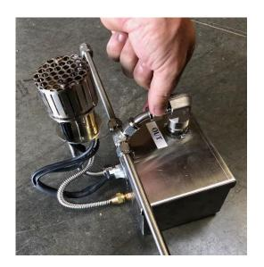
Next install the Submersible Manifold onto the outlet of the Ignition Control Box. The submersible manifold should be installed with the inlet to the manifold lower than the outlet fitting of the Ignition Control Box as shown in the photo at left.
