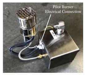
The last connection between the PBA and the Ignition Control Box is the plug-in electrical connection. The connector is a shaped connector and can only be plugged in one way. If it feels like you are exerting excessive force plugging the connector in make sure you have it oriented correctly.
