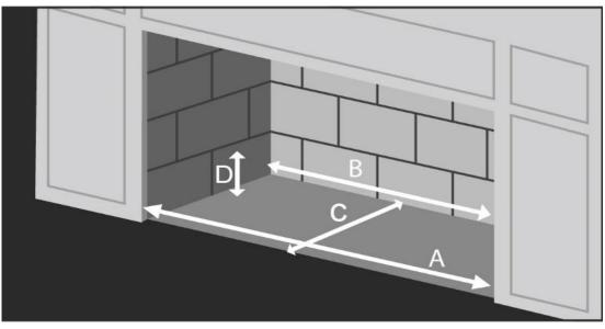
A is considered the Front Width, B is the Back Width, C is the Depth, and D is the Height.
