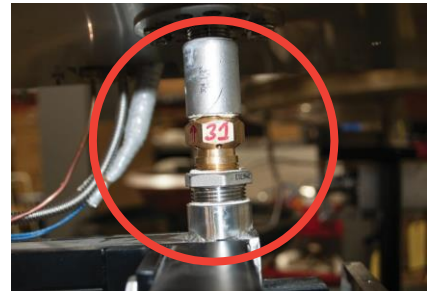
Figure 9.1 – Locating orifice for cleaning
