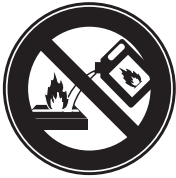
DO NOT FILL WHILE OPERATING
