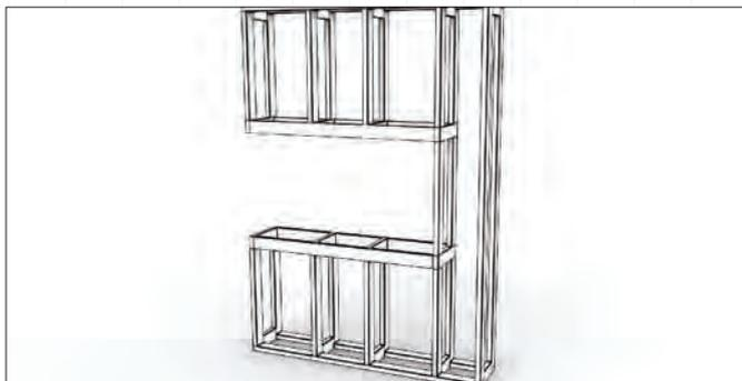
2. Slide the appliance into the framing cavity (the bottom tray can sit directly on top of the frame). The appliance is shipped with red stability bracket(s) on the open sides to keep the appliance square while in transport and during installation. Keep these brackets on while framing up the setting to assist in minimizing movement of the appliance.
