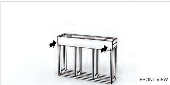
6. Complete the construction by finishing the wall paneling around the appliance. (See section on **FINISHING INSTRUCTIONS** and ensure that you fully understand where non combustible materials must be used.)
