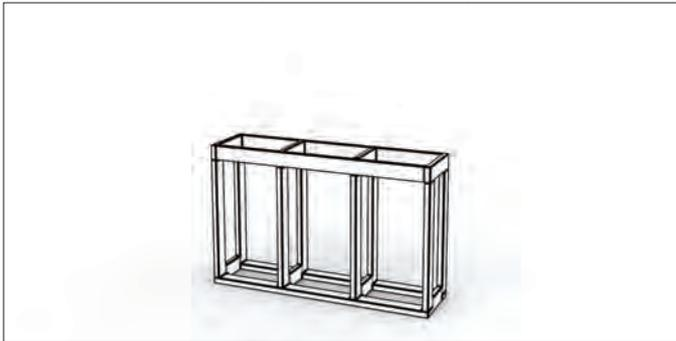
4. Align the flange extension panel with the threaded holes on the appliance. Screw it into place using the included screws (bottom row onto appliance, top row onto framing material) to secure it into position.
