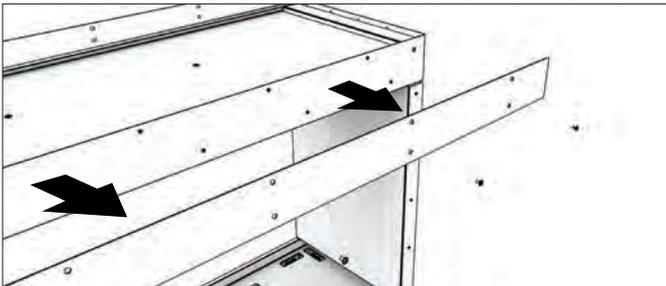
5. Fix the appliance to the framework with screws using the existing mounting holes on the appliance flanges. Make sure that the appliance is level before securing it in place.
