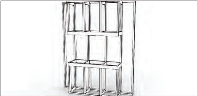
2. Slide the appliance inside the framing cavity (the base of the appliance can sit directly on top of the 2 x 4 framing material). The appliance is shipped with red stability bracket(s) installed on the open side(s) to keep the appliance square while in transport and during installation. Keep the bracket(s) on while framing up the setting to assist in minimising movement of the appliance.
