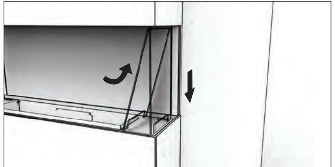
11. Install the windscreen by inserting the two ends into appropriate slots in the appliance. Use a small amount of pressure to push the windscreen in place until it bottoms out into the hidden glass clips.
