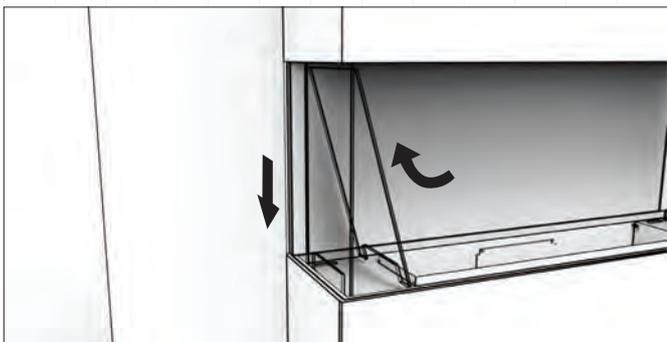
10. Install the windscreen by inserting the glass ends into the slots. Use a small amount of pressure to push the windscreen in place until it bottoms out into the hidden glass clips.
