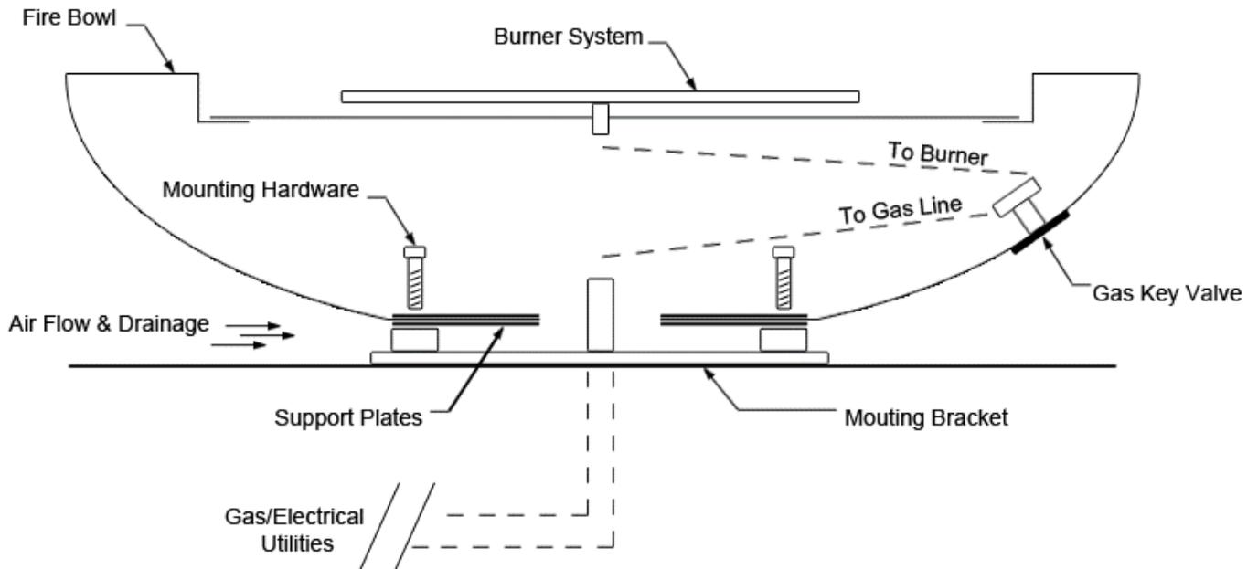
1. Place **Mounting Bracket** over **Gas/Electrical Utilities** and mark where the holes are.
