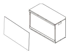
3. Pour the media into the tray. Feel free to use any combination of the fire glass media that you find most appealing. Insert the front glass panel back in place after the media installation has been completed.
